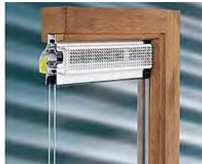
Figure 3 - 17. Outdoor grille with silencer, integrated in window frame. For natural air supply in case of mechanical exhaust systems (system "C")
