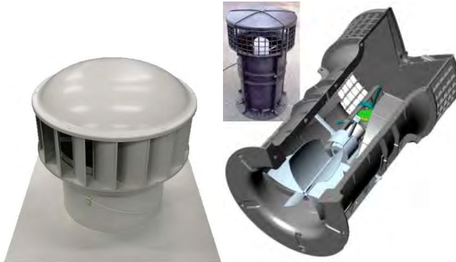
Figure 5- 8: Two examples of centrifugal fans for intermittently fan-assisted stack ventilation. The left hand cowl has SFP \approx 1 , and a discharge coefficient of 0,51 < CD < 0,81 ( 1,5 < \xi < 3,7 ) when free-wheeling. The right hand fan has negligible pressure drop when switched off and SFP \approx 0,19 at 10 Pa & 42 \ell/s with 8 W DC-motor fan with system efficiency 5,2%. Peak system efficiency is approx. 6,5% [source: CSR Edmonds; Aereco]
